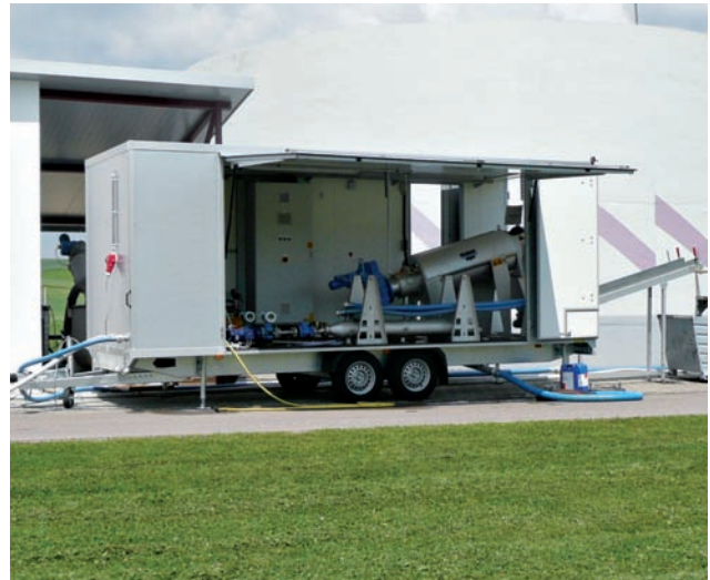
Mobile unit mounted on a trailer
