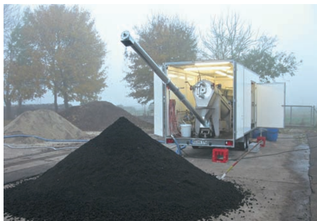
Mobile RoS 3Q 440 unit for contract dewatering
