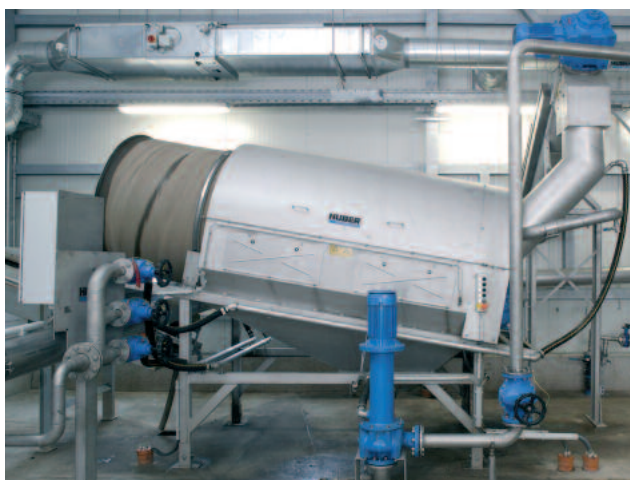
ROTAMAT® Wash Drum for washout and separation of all coarse material > 10 mm
