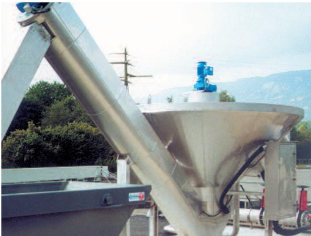
*Innovative technology: COANDA Grit Washer RoSF 4 size III with frost protection for outdoor installation*
