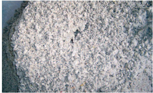
*Particularly hairs and fibres are separated by means of the two-dimensional square mesh design.*
