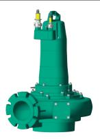
FK motors feature an oil-filled motor chamber. By means of an internal oil circulation cooling system, the heat produced by the motor is dissipated to the pumped media via a heat exchanger. The type FK 17.1 of this series is available in explosion-proof design. Advantages:
