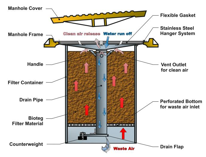
Odorous air from the sewage system enters the biofilter through its perforated bottom.
